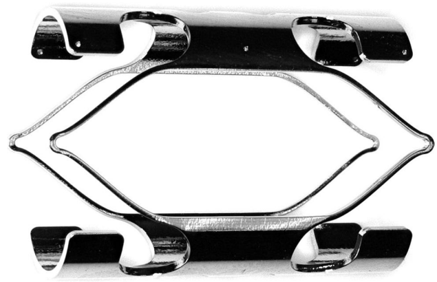
Fig. 1 As as-manufactured “double diamond” Nitinol coupon specimen
